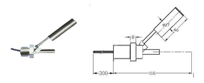
**Operation:** When the float drops to the horizontal position, the internal reed contacts draw together and complete a circuit. When the float rises from the horizontal position, the contacts separate and open the circuit.
