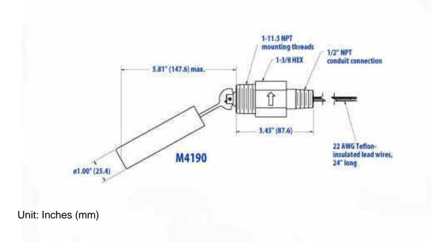
**Operation:** When the float drops from the horizontal position, the internal reed contacts separate and open a circuit. When the float rises from the horizontal position, the contacts close and complete the circuit.
